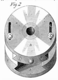
equally as well as to new ones, and will add only from one to one and a half inches to the depth of the entire chuck, including the attachment. Although only one sliding plate is represented in this engraving, says the inventor, another slide can be added if necessary.
