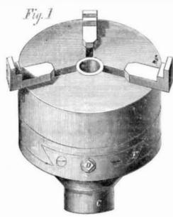
or cams, and it is to be applied particularly to scroll chucks, which are arbitrary in their motions and cannot be set out of the center unless one of the jaws be taken out and started on the thread after the other jaws have been run in one turn or two. Even this will not always bring the work true, and some simple arrangement of the kind here shown will prove a
