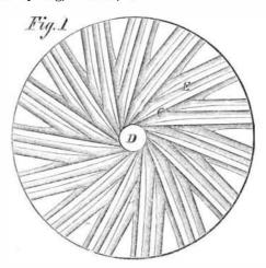
"My improvement has a two-fold object, viz.: to effect the grinding as near to the eye as possible, thereby saving the power required for driving the stone, and by so doing to carry off the flour in the furrows and prevent its keeping between the lands of the stone as it approaches the periphery, whereby overgrinding is produced from greater friction, and retention of the flour between the parts of the stone that revolve the most rapidly.
