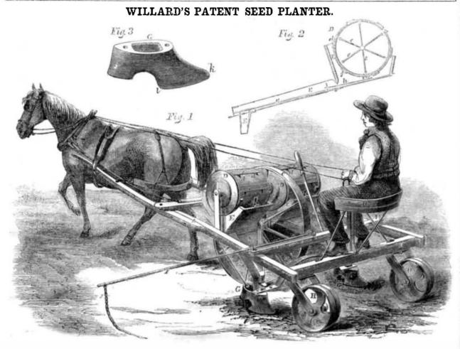
The advantage of this seed planter over the | numbers that are in operation is shown and will be understood from the following description and engravings, of which Fig. 1 is a perspective view of the whole, Fig. 2 a section of the seed-planting device, and Fig. 3 an enlarged view of the furrower and presser.
