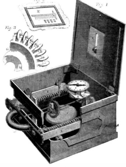
This is an instrument for ascertaining and registering the draft of plows, mowers, reapers, wagons, carriages, &c., and, as its name signifies, it is a measurer of motive power.
