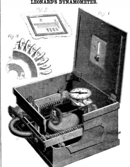
This is an instrument for ascertaining and registering the draft of plows, mowers, rcapers, wagons, carriages, &c., and, as its name signifies, it is a measurer of motive power. At the present time, when every State and
