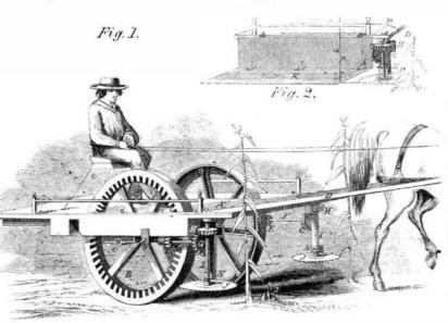
J J, are hung, supported by the iron brace, (not seen in engra ving), placed under the N, fastened firmly to the under side of frame- | platform. P P are rods for guiding the cut work. D are the shafts. corn on to the plate or bed, K, and also for
