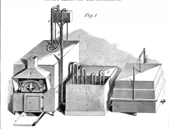
ties. Then passing up the pipe, G', it arrives at the box which represents the hydraulic main. In our illustration this has been turned one quarter round, so as to show the | 1. The gas them passes through the water, e, internal arrangement of its parts. The gas passes through the small box, d, becoming cooled and leaving behind, it its tar until there | into the condensers I, placed in a tank of water,
