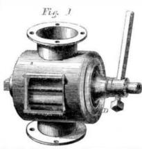
throttle, in the event of the strap of the governor breaking, thus preventing the damage which usually follows such an accident.
