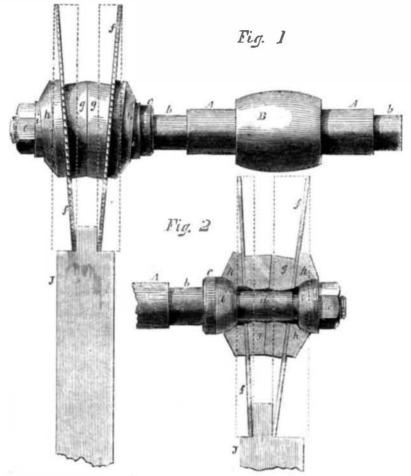
be least when the thinnest parts of the washers are brought into coincidence. In addition to the thickness of the tongue, the relative obliquity of the saws to the axis of the spindle can, by means of the washers, h h, and rings, ii, be made such that one saw will stand more oblique than the other, thus admitting
