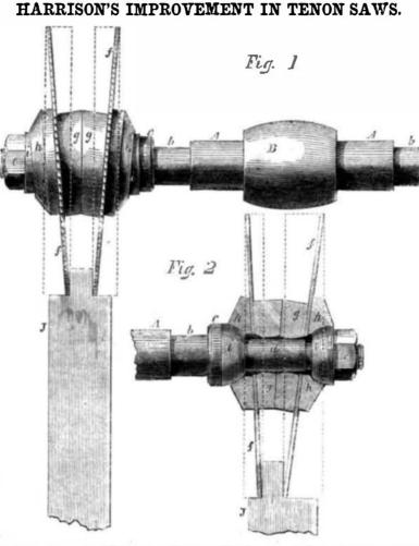
position of the two interior washers, and will of the tongue as regards the end of the stuff, be least when the thinnest parts of the washers are brought into coincidence. In addition to the thickness of the tongue, the relative obliquity of the saws to the axis of the spindle can, by means of the washers, & h, and rings, i i, be made such that one saw will stand more oblique than the other, thus admitting of the cutting away of more wood on one side Philadelphia, Pa. Patented July 14, 1857.
