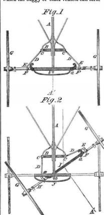
Fig. 1 shows the perch and front axle of a buggy when straight, and Fig. 2 shows the same when turning a curve, the lines, A A',
