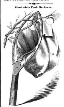
A great quantity of fruit is spoiled in the gathering, by being allowed to drop on the ground, or else the tree is much injured when they are violently pulled off by hand, as the small branches are liable to be broken. This simple little device, cheap and light, is one of the best we have seen for gathering fruit, neither spoiling it or damaging the tree. Any child can use it, and every one who gathers fruit should.
