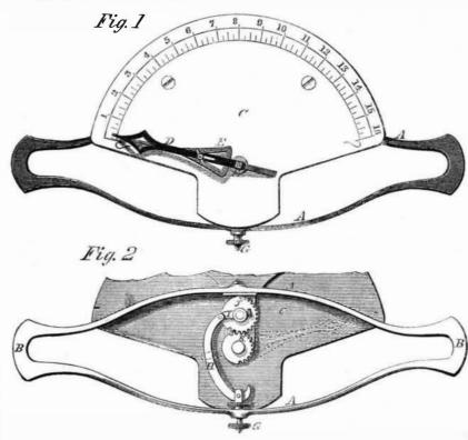
course, causes the pointer, D, to move round | tion, and is manufactured, or the patent is for the dial, and the whole being proportioned and graduated correctly, the indicator, E, being only loosely placed on the axis, F, vibrates as the implement to be tested is drawn along, and indicates the average draft very
