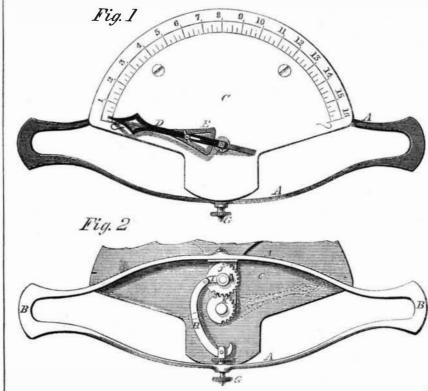
course, causes the pointer, D, to move round | tion, and is manufactured, or the patent is for the dial, and the whole being proportioned and graduated correctly, the indicator, E, being only loosely placed on the axis, F, vibrates as the implement to be tested is drawn along, and indicates the average draft very accu rately.
