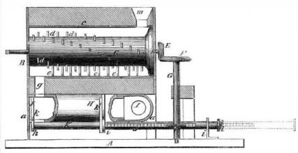
This machine makes sausages direct from stationary metal plates, e. These plates are gitudinal section through the invention, A is the meat at one operation, without any all parallel with each other, and equal dishandling or chance of uncleanly treatment. Our engraving is a transverse vertical section of one of these machines, which the following description will explain :-
