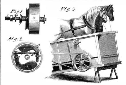
subject of the accompanying illustration is designed to regulate the speed of horse powers. and keep the fly wheel rotating at an equal and regular rate.
