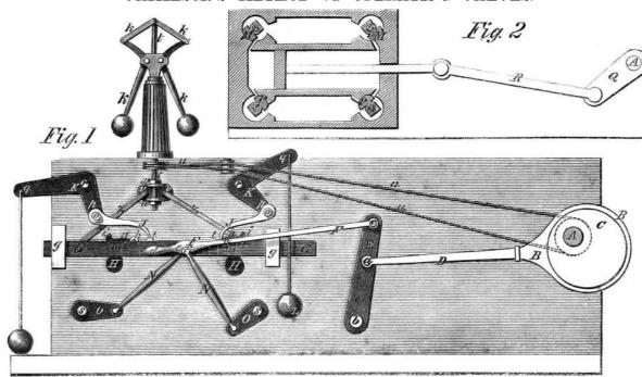
it is so light, being merely to depress the end of the swinging dog, that the governor is not affected in its regular motion thereby, as it would be were any of the parts bearing or
