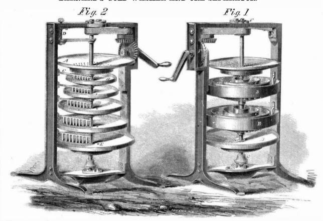
of the pan to the one below, which is made broader, to receive it, and so on to the next in order, till it passes to the bottom pan, E, the gold being retained in the upper ones. In each of these pans is a hole closed with stoppers, which can be removed to allow the gold
