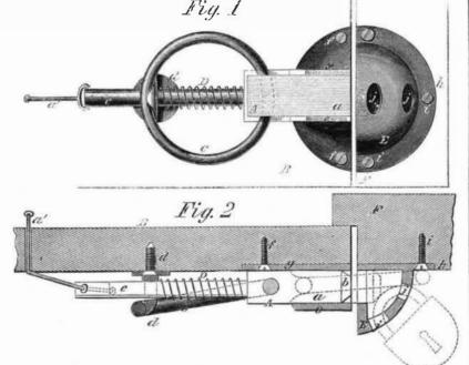
slide bolt, with a ring attached, employed in connection with a spring, socket or nosing and guide, so that a most simple and economical ring bolt is obtained, which is suitable for the ordinary hinged doors or sliding ones, such as railroad freight cars, where they should be placed vertically, the socket being in the floor or in the top, as most convenient, and not horizontal as in our illustrations.
