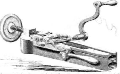
ELMER'S MACHINE FOR GUMMING SAWS.
