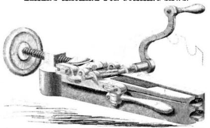
held perfectly firm that it may be cut quite true, and the cutting tool should be of such construction that it will fairly cut away the metal and not tear it. The machine for filing, gumming and jointing saws (of which
