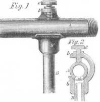
When gas or water pipes are laid, much time and labor are expended, and consequent expense incurred in joining the branch pipes to the main, and in connecting the supply pipes to the branch. The branch pipes are usually cut in two, their ends are then cut
