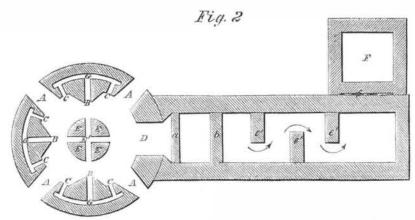
places, every portion of the fuel has a chance of being burned. The heated products of combustion pass through the flue, D, and over the bridge, b, giving up their heat to the boiler, and also in the direction of the arrows in Fig. 2, around the side bridges, e', so that no heat may be lost. There is a damper, f, at the side of the chimney, which directs the as above.
