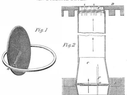
A great objection to the use and adoption of air-heating furnaces is that the hot air conducting pipes are very liable to become overheated when the registers are closed; and from this cause many serious accidents have
