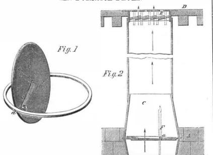
them consequently stopped, the dampers will close by their own gravity, and shut off the pipesfrom the air-heating chamber; and when the registers are fully, or more or less open, the dampers will be opened to a corresponding degree by the action of the draught.
