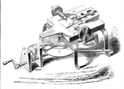
vention in this mortiser are, the peculiar methods employed of giving the feed motion to the cutters, and other points, that will be seen as we proceed in our description. It is a supplemental machine to the above, and can either be used as such or by itself, the hubs being turned by any other machine. It was patented this week, and the claim will be found on another page.
