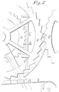
projection, k, and working up and down in suitable bearings; there is also a spring, 1, which has a tendency to force the bar, K, up and keep it from the bricks.
