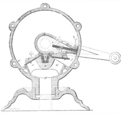
This pump can be worked by hand for wells, &c., or by power, as it is peculiarly adapted to be worked by an oscillating engine, no gearing being necessary, and as a fire engine it would be valuable. They can be 24, 1857.
