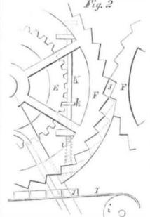
projection, k, and working up and down in suitable bearings; there is also a spring, l, which has a tendency to force the bar, K, up and keep it from the bricks.
