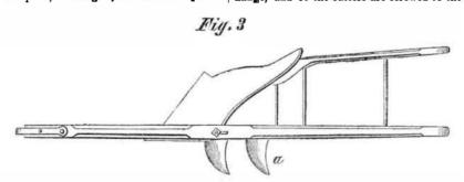
plow. There is a slot in the landside of the | entirely when necessary, as when plowing plow, through which the cutter is passed, and the bolts are put through the side of the plow, and passed through the flange inside. By taking off the bolts, the cutters are easily removed for sharpening, and they can again
