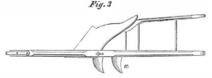
plow. There is a slot in the landside of the | entirely when necessary, as when plowing plow, through which the cutter is passed, and the bolts are put through the side of the plow, and passed through the flange inside. By taking off the bolts, the cutters are easily removed for sharpening, and they can again be easily attached, or they can be removed any further information that may be desired.
