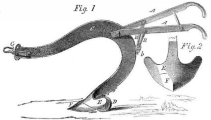
The adaptation of the plow to cultivating, as well as turning up the ground, is a valuable application ; and those plows which break up the ground without leaving a furrow, are called from their shape, "shovel plows." They are used for cultivating cotton and sugar, and sometimes, when the ground is light, for breaking up, as in the sandy soil of South Carolina.
