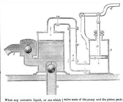
has a tendency to oxydize, to abrade, or eat away, the surface of metal (or, in fact, any substance of which pumps are usually constructed) has to be raised, the operation is | liquids, and is so arranged that the liquid always difficult and expensive, because the | never comes in contact with the pistons, but
