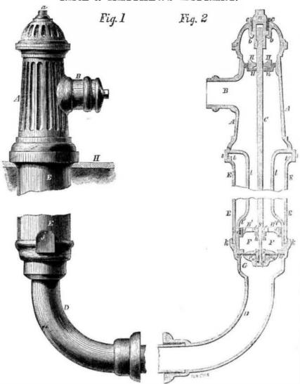
The chief features of novelty in this hydrant are that, by the peculiar arrangement of the valve, the waste pipe is opened as the induction pipe is closed, and it can be readily removed from its base without the necessity of excavating.
