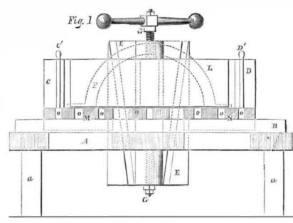
plate, E, and turning the screw, G; when the tire is clamped, the screw is turned in the opposite direction, and raising the block, E, forces together the blocks, C D, thus compressing the tire, or as it is technically called upsetting it. Straight bars can be upset, as
