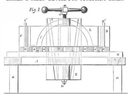
plate, E, and turning the screw, G; when the tire is clamped, the screw is turned in the opposite direction, and raising the block, E, forces together the blocks, C D, thus compressing the tire, or as it is technically called upsetting it. Straight bars can be upset, as
