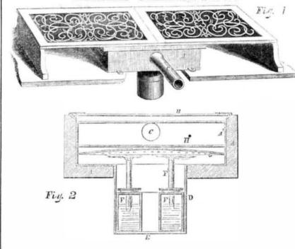
John W. Lefferts, of Brooklyn, N. Y., is the inventor of the simple means here represented for providing a source of heat, by which the feet may be warmed in sleighs or other vehicles. This stove, as it may be very properly termed, is inserted in the bottom of the vehicle, a principal portion being below the ordinary floor. Fig. 1 is a perspective view, and Fig. 2 a vertical section.
