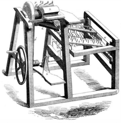
placed in the groove of A, with the butt towards the knife, F, and projecting just sufficient to be cut off; it is held in its place by the springs, E. It then passes into G, which delivers it on the platform, I, where the husk is torn off by the combined action of the sharp rake teeth and the motions of the platform and rake, and the corn turned out ready for shelling.
