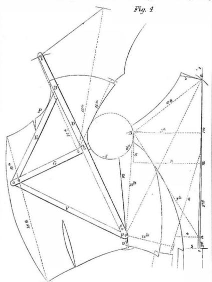
care to bring the pivot, d, opposite the middle of the place where what is termed the "back seye" ought to be, then by turning the set screw, b, the hoop will be fixed to the right size. Suppose, for example, that the instru-
