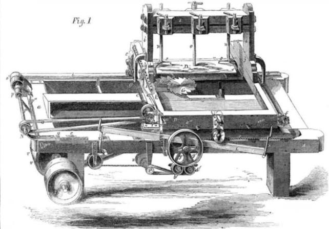
bar, L, vertical guides, j, are secured (seen in vertical section in Fig. 3) and between these guides a slide, k', is placed, this slide having a roller, l', at its lower end. A pin, m', is also attached to the lower end of k', which fits into a slot in L.
