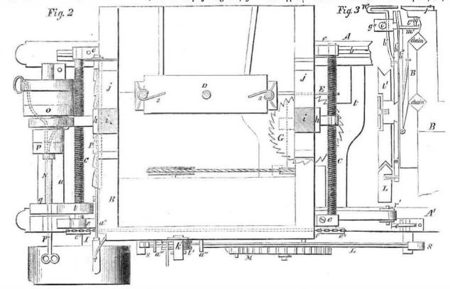
out by a small spring in the back of it, and is drawn in by a short arm, l", working in a staple or hook, m'', attached to pawl, k'', said arm, l", is attached to a small rockshaft, n, in the side of carriage, B, which
