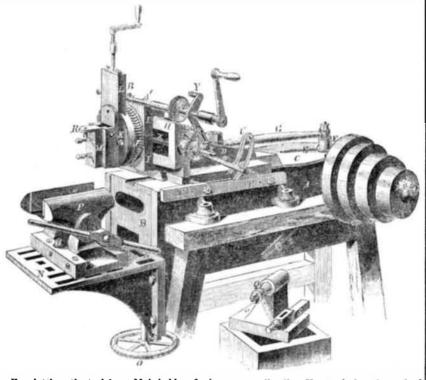
For slotting, the tool-box, M, is held as for shaping, when the slotting tool will be in a line with the working slide, D, as in an ordinary slotting machine. The work may be held either in the vice or on an angle plate bolted n the table, N.
