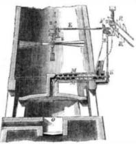
A is the cone of the glass stack or house; it is furnished with a screw fan-wheel, B, set in the wall, and revolving horizontally in the stack. The bevel gear, C D, operated by the fan, gives motion to the shaft, E, on which are gears, F G, that give motion to the vertical shaft, H, the lower end of which has a worm wheel on it that meshes into another,
