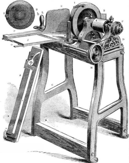
tions to any desired thickness, bevel or taper, at the rate of about thirty feet per minute, and also take the "wind" out, leaving the surface smooth, and the corners perfect. They are remarkably simple, and not liable to get out of repair.
