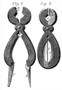
pivoted a screw-driver, F, which can also fold back when not in usc; a spring is arranged at the back of these recesses to open the pincers. The recess is so cut at the end of the long arms that it forms a step or support for the tool that is in use; the tool that is shut up leaving sufficient room for it to fit partly into its recess, so that both arms have a hold upon
