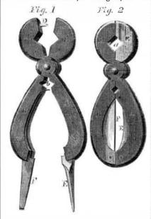
pivoted a screw-driver, F, which can also fold back when not in use; a spring is arranged at the back of these recesses to open the pincers. The recess is so cut at the end of the long arms that it forms a step or support for the tool that is in use; the tool that is shut up leaving sufficient room for it to fit partly into its recess, so that both arms have a hold upon
