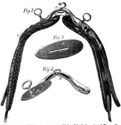
Harness trees which have to bear the weight of the shafts must be made sufficiently strong to hold up the shafts, and at the same to so adjust the weight as not in any way inconvenience or chafe the horse. The harness tree we are about to describe fulfils these conditions, but is applicable only to light carkind. It is the invention of Thomas Dempsey, of the firm of O. Macfarland & Co., harness-makers, Newark, N. J., and was patented by him Jan. 12, 1858.
