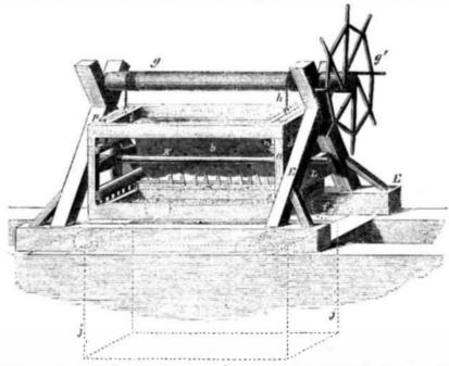
up and the frame, E, moved to the desired vat by means of the runners, f. In order that the frame may be equally balanced, in filling it, sides are put in alternately with a neck and a butt at each end.
