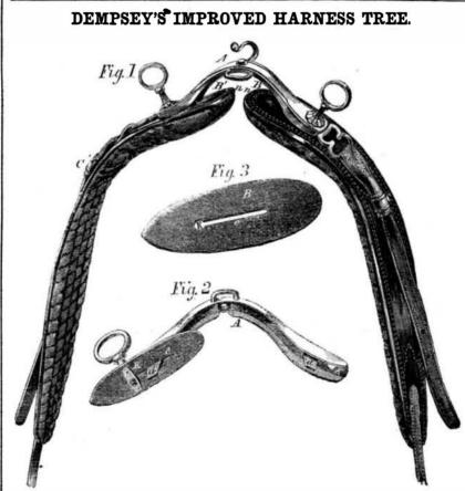
Harness trees which have to bear the weight of the shafts must be made sufficiently strong to hold up the shafts, and at the same to so adjust the weight as not in any way inconvenience or chafe the horse. The harness tree we are about to describe fulfils these conditions, but is applicable only to light carsticks, c, which are kept the proper distance | riages and coaches, and not to saddles of any | in forming a metallic tree, A, with its center
