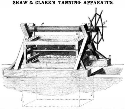
other and from one vat to another, a is drawn | tion of the gelatine, and saving of time in proup and the frame, E, moved to the desired vat by means of the runners, f. In order that the frame may be equally balanced, in filling it, sides are put in alternately with a neck and a butt at each end.
