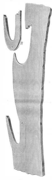
loose, for the reason that the action of them on the wood being sawed tends to bind them firmly in place, and that the greater the resistance the stiffer they become. The heveled edge of the seat on the saw prevents the tooth from slipping sidewise, as may be seen.
