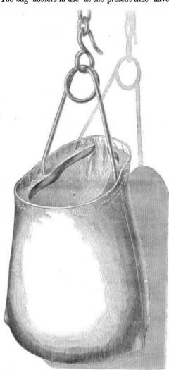
proved very handy, and that here shown seems to be a capital one. It consists of a single wire, A, bent so as to form a spring, and provided at the ends with metallic arms, B, which distend the bag, as shown; indeed, the artist has left us but little to do by way of description, so clearly are all parts, and the uses of them, shown.
