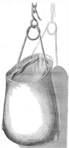
proved very handy, and that here shown seems to be a capital one. It consists of a single wire, A, bent so as to form a spring, and provided at the ends with metallic arms, B, which distend the bag, as shown; indeed, the artist has left us but little to do by way of description, so clearly are all parts, and the uses of them, shown.
