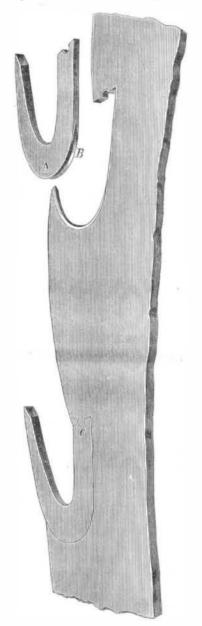
loose, for the reason that the action of them on the wood being sawed tends to bind them firmly in place, and that the greater the resistance the stiffer they become. The beveled edge of the seat on the saw prevents the tooth from slipping sidewise, as may be seen.
