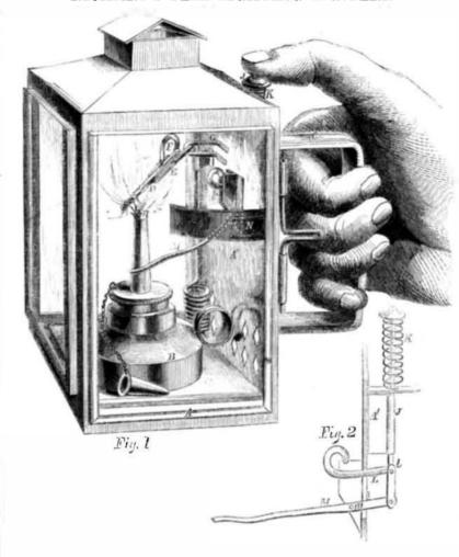
is pressed on the cap on J, and L being depressed allows the spring to pull back E, and drag the match quickly against the plate, N, which ignites it, at the same time the hooked bar, M, ascends, and its hooked end throws off the extinguisher which ordinarily covers the wick. The match then burns over the wick and ignites it, and at the same time | AMERICAN.
