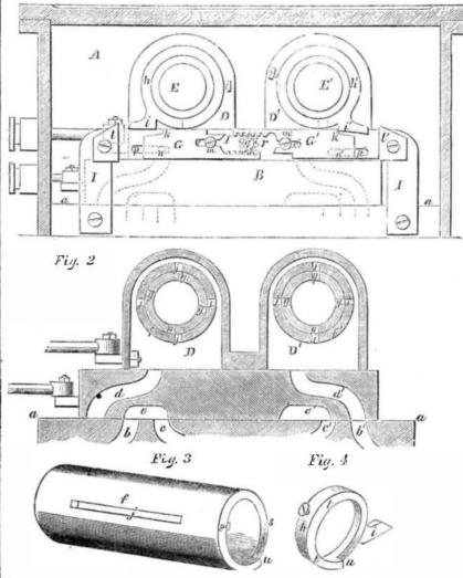
The jogs, u u, on the seats, f f', and collars, | invention of Addison Crosby, of Fredonia, N. Y., and was patented Jan. 19, 1858, from h h', serve as stops to prevent the turning of the cut-off valves further than is necessary in whom all further information can be obtained. closing.
