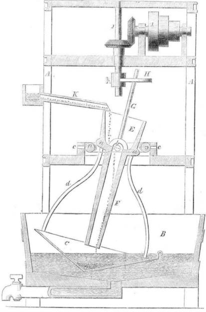
This improved ore-washer was noticed on | its motion through a pair of bevel gear wheels page 51, present volume, of the Scientific AMERICAN, and we now give an extended description, with an engraving showing a vertical section through the machine.
