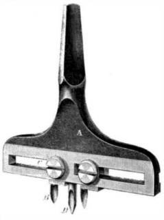
center of the casting there is a fixed point, D, which is also capable of making a hole. This tool will cut out a ring of leather of any required dimension within the range of its width; it is quickly adjusted, and always ready for use. It is also convenient for joiners and pattern makers to cut their wood into circles when needed. It is used with a common brace.
